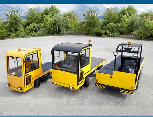
LOAD CAPACITY 2000 - 25 000 kg MOVEMENT SPEED 20 - 25 km/h
