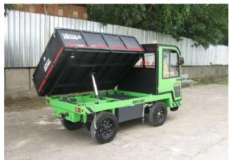
The electric dump truck is made in accordance with BDS EN 3691-1.
